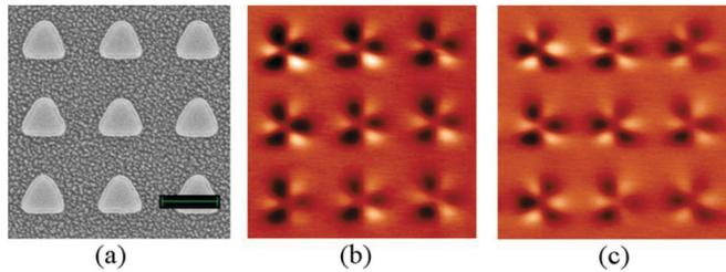
FIG. 1. (Color online) (a) Scanning electron microscope (SEM) image of the lattice of the cobalt triangles, the scale bar length is  $1 \mu\text{m}$ . (b) MFM image of the remanent states after magnetizing along the base of the triangles. All magnetic vortices demonstrate the same direction of the vorticity. (c) MFM image of the remanent states after magnetizing along the height of the triangles. The vortices with both CW and CCW vortices are presented.
