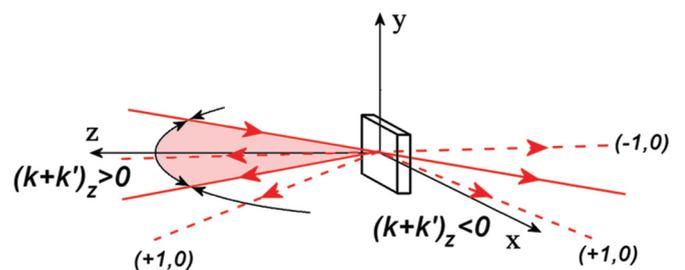
FIG. 3. (Color online) The geometry of the experiment. Solid lines are incident, transmitted, and specularly reflected beams, dashed lines represent diffracted beams. The gray-colored (red online) segment of the  $XZ$  plane corresponds to the directions with  $(k + k')_z > 0$ .
