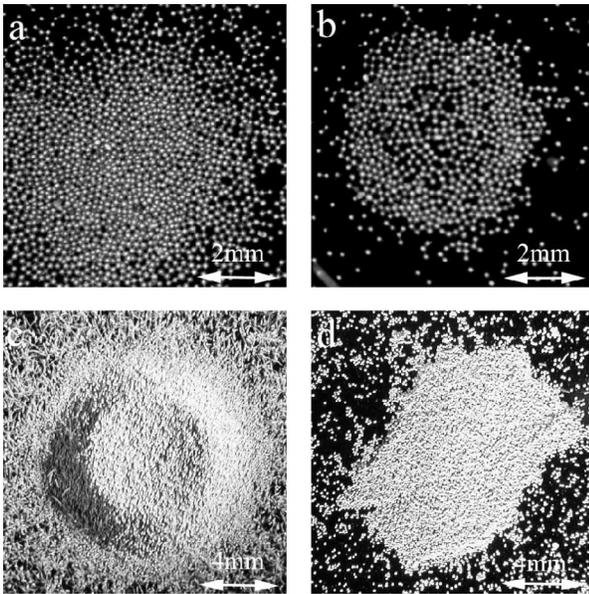
FIG. 1. Shapes of granular clusters. Upper row shows clusters in electrostatically driven system. (a)  $f=20$  Hz; (b)  $f=120$  Hz. Bottom row shows clusters in mechanically vibrated system. (c)  $f=25$  Hz; (d)  $f=95$  Hz. Left column: heaplike clusters corresponding to 3D behavior. Right column: flat monolayer clusters corresponding to 2D regime.
