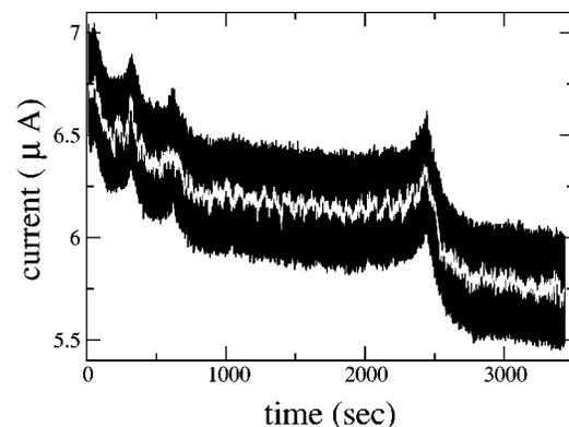
FIG. 5. Current vs time during coarsening in dc electric field. White line shows the signal averaged over 100 points. Current peaks correspond to evaporation of clusters. The signal/noise ratio is greater than 3.
