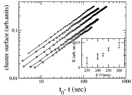
FIG. 4. Cluster area vs time for electrocell.  $f = 20$  Hz. Circles: electric field  $E = 230$  V/mm. Squares:  $E = 240$  V/mm. Diamonds:  $E = 245$  V/mm. Triangles:  $E = 250$  V/mm. Crosses:  $E = 260$  V/mm. Inset: the dependence of cluster surface tension on the applied electric field.
