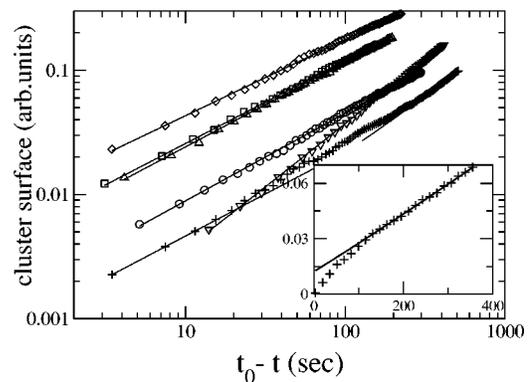
FIG. 3. Cluster area vs time for electrocell. Circles:  $f=0$ ,  $\beta=0.7$ . Squares:  $f=10$  Hz,  $\beta=0.67$ . Diamonds:  $f=20$  Hz,  $\beta=0.63$ . Up triangles:  $f=50$  Hz,  $\beta=0.68$ . Crosses:  $f=75$  Hz,  $\beta=1.04$  at the initial stage of evaporation (see inset) and  $\beta=0.67$  at the end. Down triangles:  $f=100$  Hz,  $\beta=1.02$ . Inset:  $S$  vs  $t$  for  $f=75$  Hz in linear scale.
