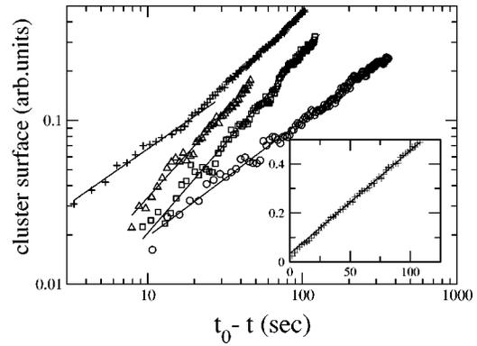
FIG. 2. Cluster area vs time for mechanical system. Circles:  $f=25$  Hz,  $\beta=0.7$ . Crosses:  $f=35$  Hz,  $\beta=1.03$  at the beginning of evaporation (see inset) and  $\beta=0.66$  at the end of collapse. Triangles:  $f=55$  Hz,  $\beta=1.04$ . Squares:  $f=85$  Hz,  $\beta=0.7$ . Inset:  $S$  vs  $t$  for  $f=35$  Hz in linear scale.
