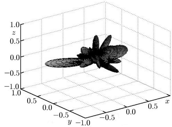
Fig. 8. Radiation pattern of the simulated Josephson antenna for a bias voltage of 0.34 V corresponding to the maximum power of the supercurrent shown in Fig. 7. A well-pronounced asymmetry of the radiation in the direction of the  $x$  axis is indicative of the traveling-wave regime. The multi-lobe character of the pattern is due to a large (compared with the radiation wavelength) size of the antenna.
