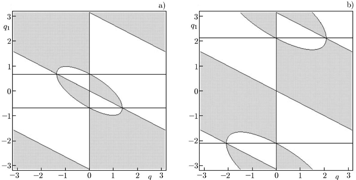
Fig. 2. Regions of stability and instability of the traveling-wave regime on the plane  $(q, q_1)$  for  $\omega_{Jd}/v = 0.3\pi/2$  (a) and  $\omega_{Jd}/v = 1.3\pi/2$  (b). The wave impedance of the line is equal to  $z_w = 4$  and the loss, to  $\nu/v = 0.01$ . The horizontal lines mark the wave numbers of the stable solutions of the traveling-wave type. It is seen that as the parameter  $\omega_{Jd}/v$  increases, the wave number of the stable traveling wave also increases.
