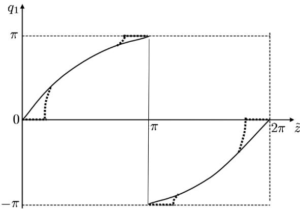
Fig. 3. Dependence of the wave number  $q_1$  of the traveling wave in the stable regime on the dimensionless period  $\tilde{z} = \omega_J d/v$ . The dotted lines show the distortion of the dependence  $q_1(\tilde{z})$  and appearance of purely in-phase and purely anti-phase regimes due to inclusion of inductive short-circuits, which make the transmission line periodic, with finite forbidden bands, even in the absence of the Josephson junctions.
