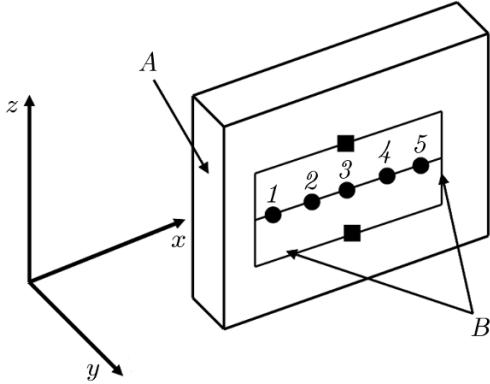
Fig. 5. Scheme of the simplest Josephson antenna in the form of a straight wire with included Josephson junctions 1–5 located on the dielectric plate A. The circles show and the squares show the power supply batteries and the Josephson contacts, respectively. The perfect conductors are denoted by the symbol B. The used systems of coordinates is also shown.
