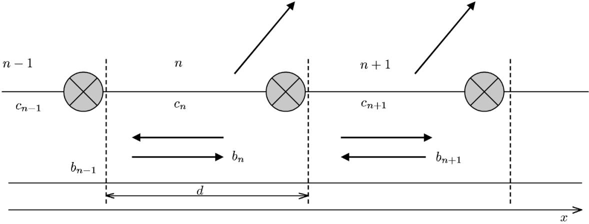
Fig. 1. Josephson junctions (shown by crosses) placed in a homogeneous line and forming a periodic structure. The arrows shows schematically the waves traveling in the line and radiating to free space. The dashed lines separating the neighboring periods mark the points of joining the current and the voltage in the line.
