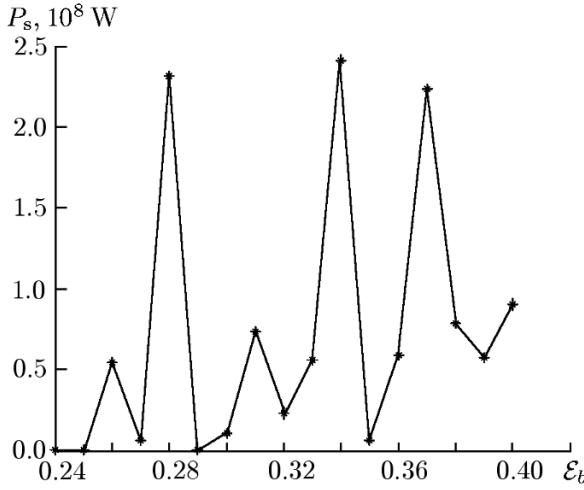
Fig. 7. Total power  $P_s$  of the supercurrent, which characterizes radiation to free space, as a function of the bias voltage. Great ruggedness of the curve on the plot is due to a strong dependence of the electrodynamic coupling parameters and the coupling conditions on the frequency.
